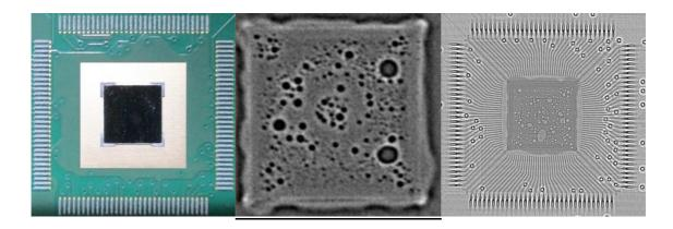
Voiding has been reduced significantly. By using preforms the assembly process can get safer and more reproducible.
