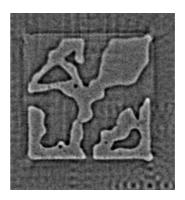
Trying to solve the voiding problem by adding more solder paste can lead to lifting of the component and problems soldering the side pins. Also, more solder paste inevitably leads to more flux/air bubbles on the exposed pad because it gets trapped and can't flow off.
